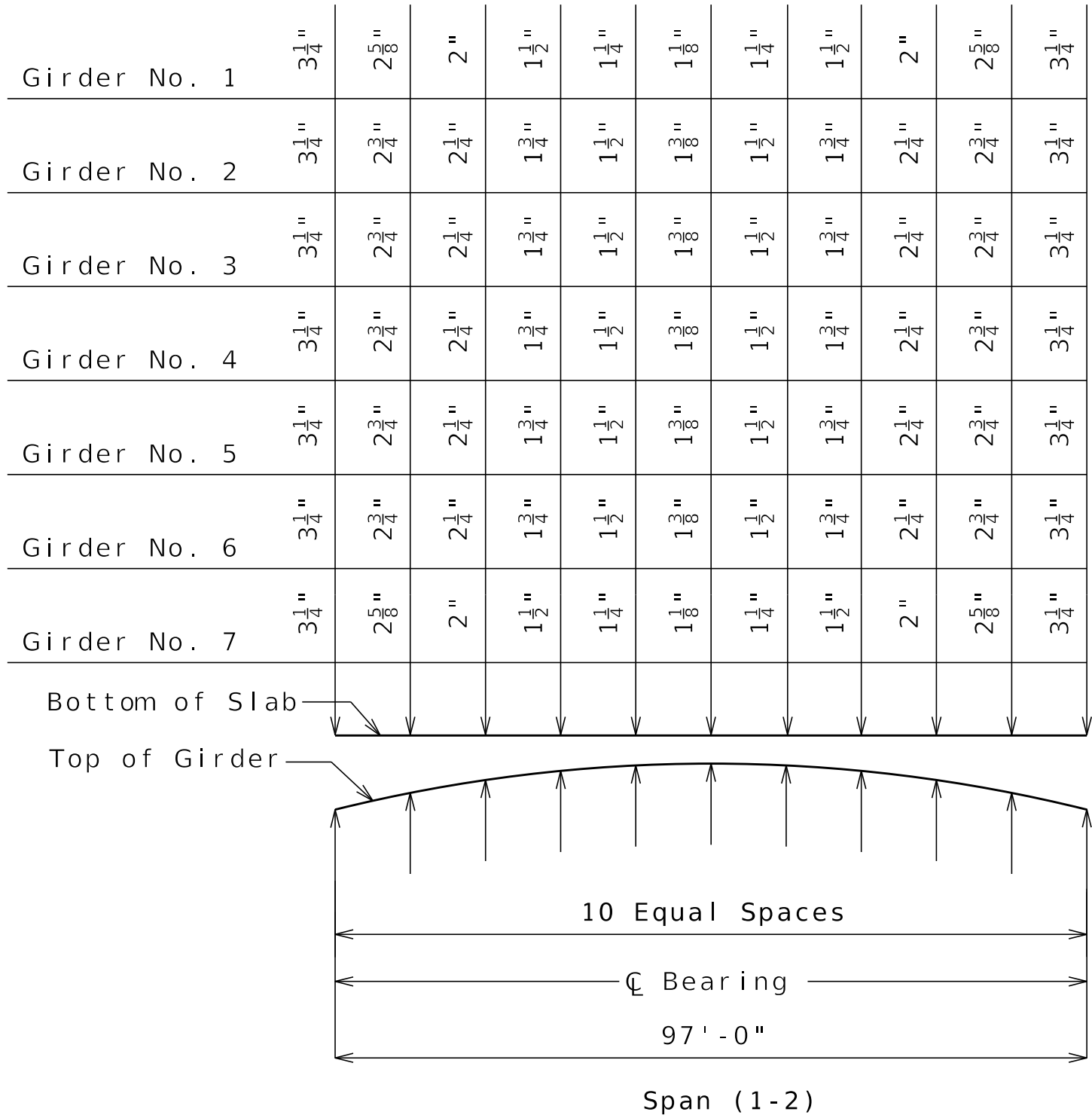
THEORETICAL SLAB HAUNCHING DIAGRAM (ESTIMATED AT 90 DAYS)
