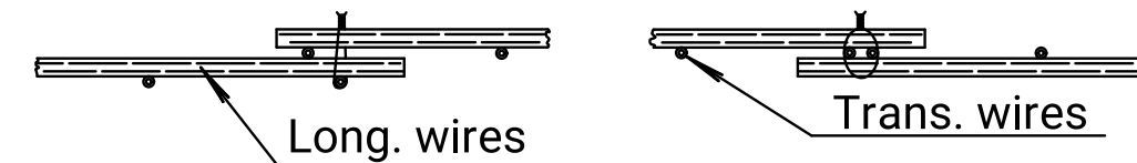
DETAIL OF LAP FOR WELDED WIRE REINFORCEMENT
