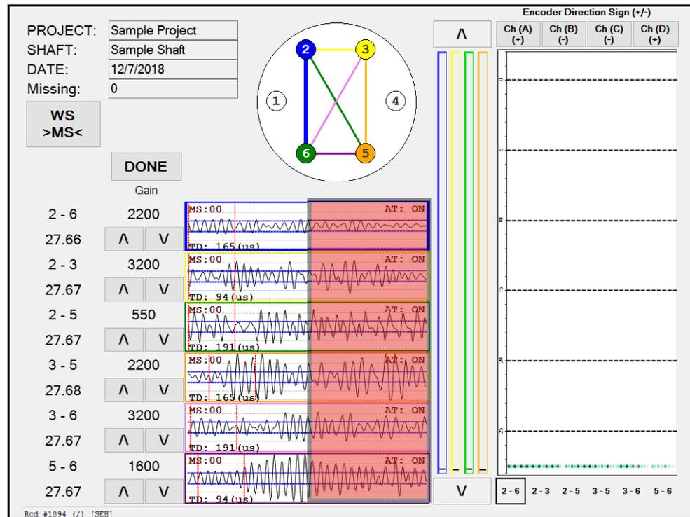
**Figure 4.11:** The AT lines for each profile may be toggles on or off.
