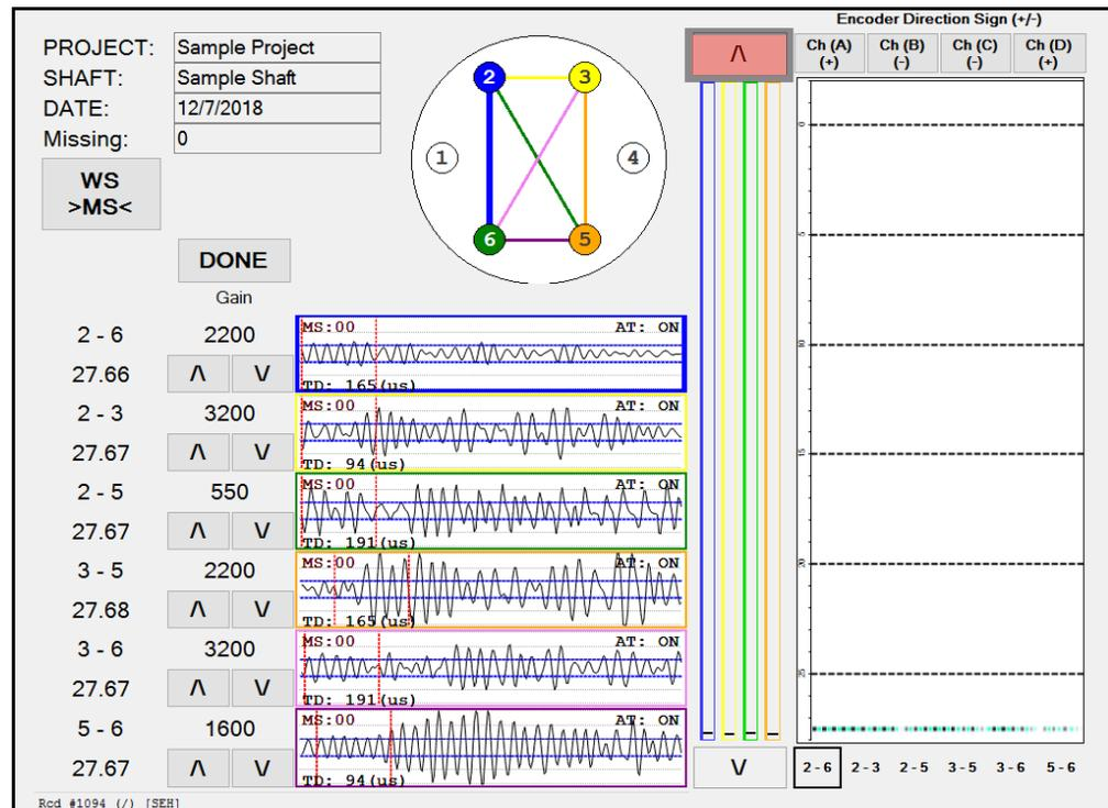
**Figure 4.4:** Zeroing the Depth Encoders at the top by selecting the up arrow (highlighted in red).
