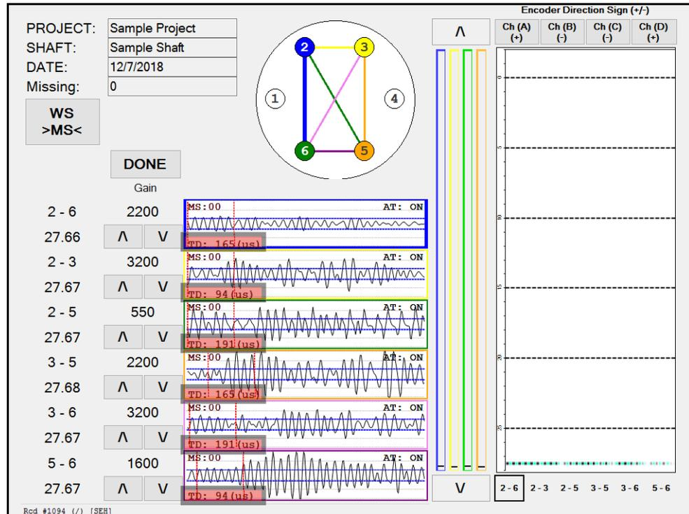
**Figure 4.5:** The Time Delay (TD) is noted in the red shaded area for each profile.
