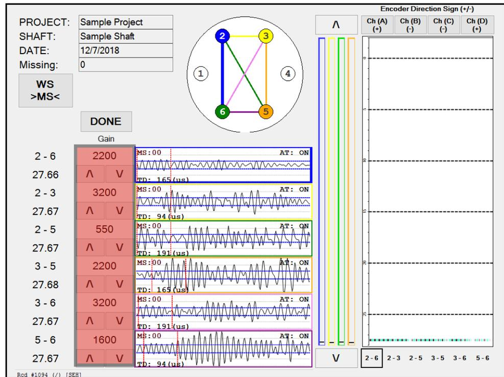
**Figure 4.6:** The Gain setting for each profile can be adjusted at the beginning of data collection by selecting the up or down arrow below each gain value (highlighted in red).
