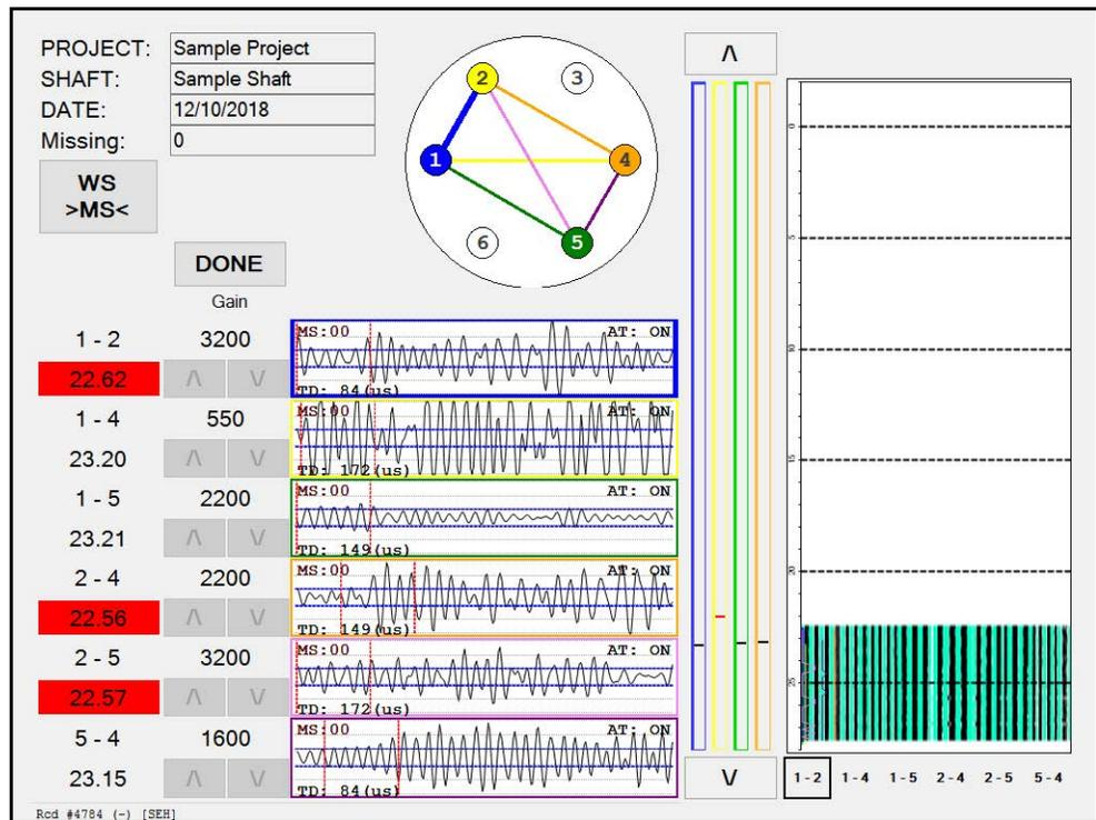
**Figure 4.8:** Probes that have a depth greater than 6 inches (15 cm) from the lowest probe will be marked in red and the associated profiles with that probe will also be highlighted in red.
