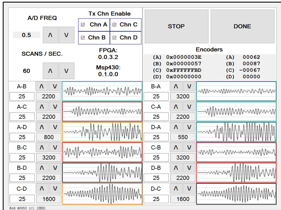
The hardware monitor allows the user to run the probes and view the signal from all probe combinations. This can be to verify that all transceiver probes are able to transmit and receive a signal. Additionally the user has the ability to adjust gain levels to determine the appropriate gain level for each profile.
