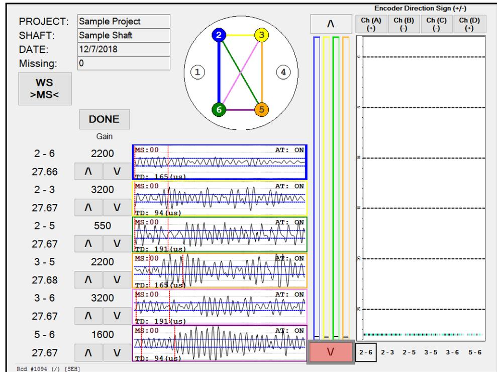
**Figure 4.3:** Zeroing the Depth Encoders at the bottom by selecting the down arrow (highlighted in red).
