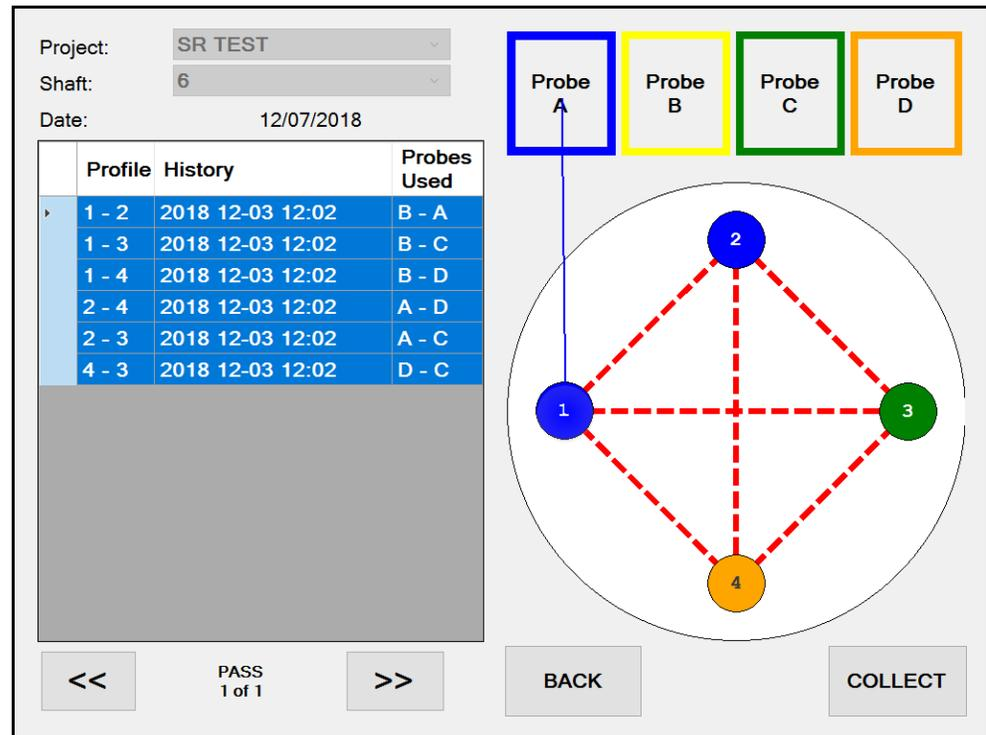
**Figure 3.10:** The Profile Selection Screen allows the user to choose which profiles will be tested by assigning probes to access tubes.
