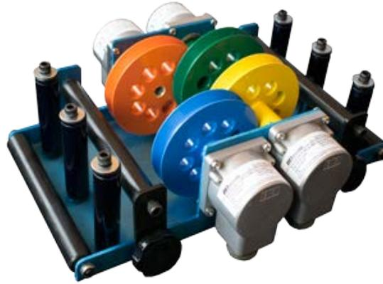
**Figure 2.8:** 4 probe tripod depth wheel encoder assembly.
