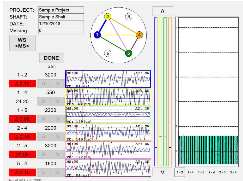
**Figure 4.9:** The depth display can be toggled to show the difference between the two probes by touch the depth value.
