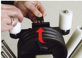
13a - Squeeze latch spring and rotate pinch rollers at the same time as shown
