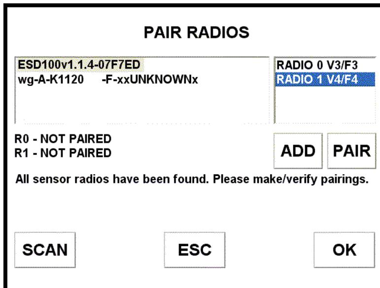
In this case the user wanted to set the gages connected to transmitter "07F7ED" to Radio 1,
