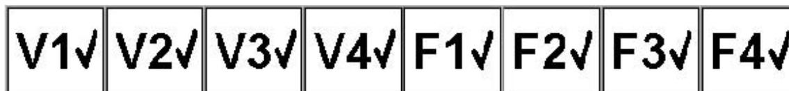
NOTE: The V1, V2, V3, V4, F1, F2, F3 and F4 buttons will appear or not depending on the PAX model (4 or 8 channels) and on the choice made on the Settings Menu (which can be reached from the Main Menu - see page 85).
