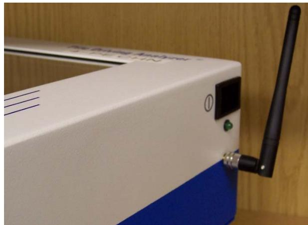
The radio transmitters can be used with the new “smart gages”. These gages will send serial number and calibration data to the PAX, so the user is no longer required to enter this information manually. This greatly reduces the risk of errors during data collection. Currently the smart gage functionality is only available with the radio transmitters. The smart gages will work with standard cable transmission, but the serial number and calibration number information has to be entered manually.
