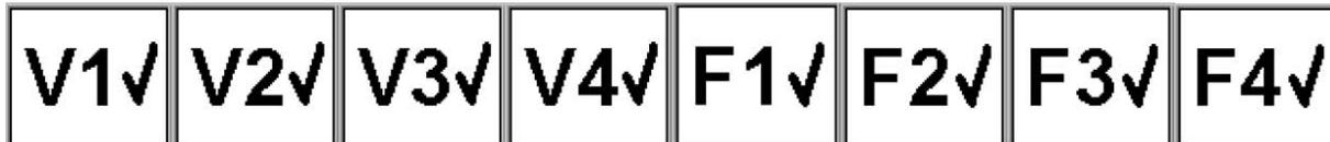
Some buttons may not be present depending on the number of gages selected in the Main Screen. Touching any button will toggle the sensor On or Off. The buttons as shown above indicate that all sensors are ON. If for instance V1 is turned OFF the corresponding button will look like this:
