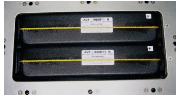
Cover removed, exposing 2 Lithium Ion batteries (Domestic Usage)
