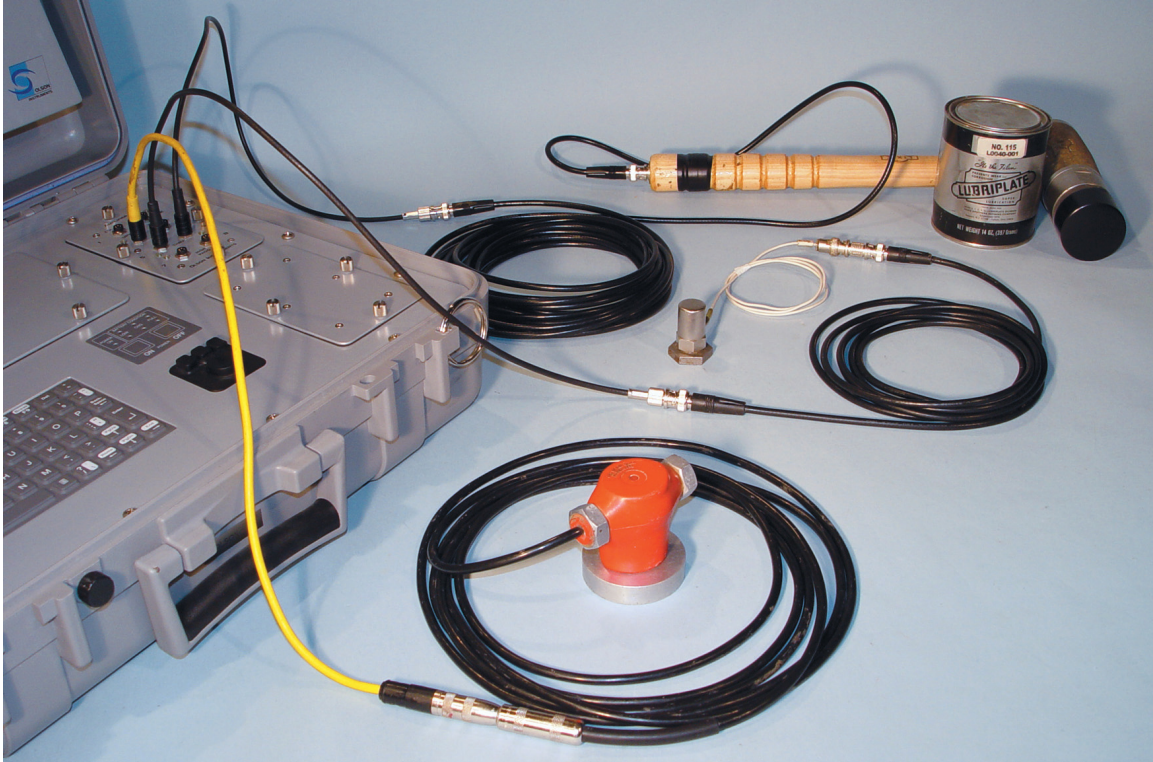
Complete SE/IR System with Accelerometer showing all components properly attached
