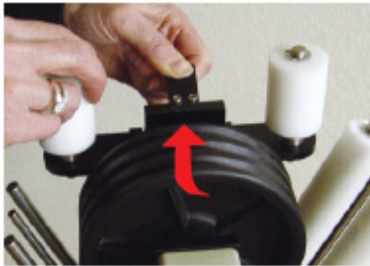
13a -Squeeze latch spring and rotate pinch roller assembly upward at the same time, as shown.
