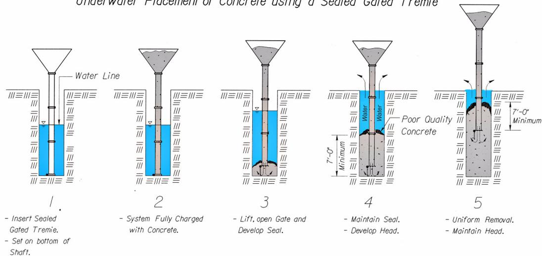
**Method 'C' (Figure 3)** uses a tremie pipe with a seal on the end, which is lowered into the drilled shaft. The seal prevents water from entering the pipe and mixing with the concrete. The tremie may have a vent tube to reduce the possibility of an air bubble being trapped in the tremie. The tremie is charged completely with concrete and then lifted off the bottom one tremie diameter to start the flow of concrete into the shaft.
