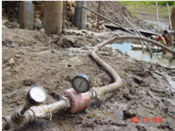
Inline Flow Device (meter): This is used to measure the volume of grout passing by a point in the grouting system.
