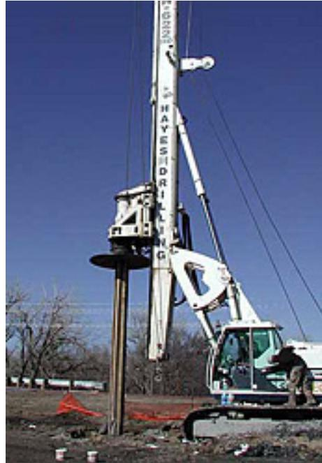
Modified Excavator Drill Rig
