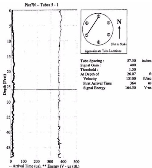
In performing the sonic logging, the probes are lowered into the CSL pipes and then raised simultaneously using a tripod at a rate not to exceed 1'-0" per second. Any sudden lengthening of the arrival time and a simultaneous drop in the energy may be an indication of poor quality concrete. This is where the concrete curves discussed above may be useful in identifying any areas in the shaft that could have problems.
