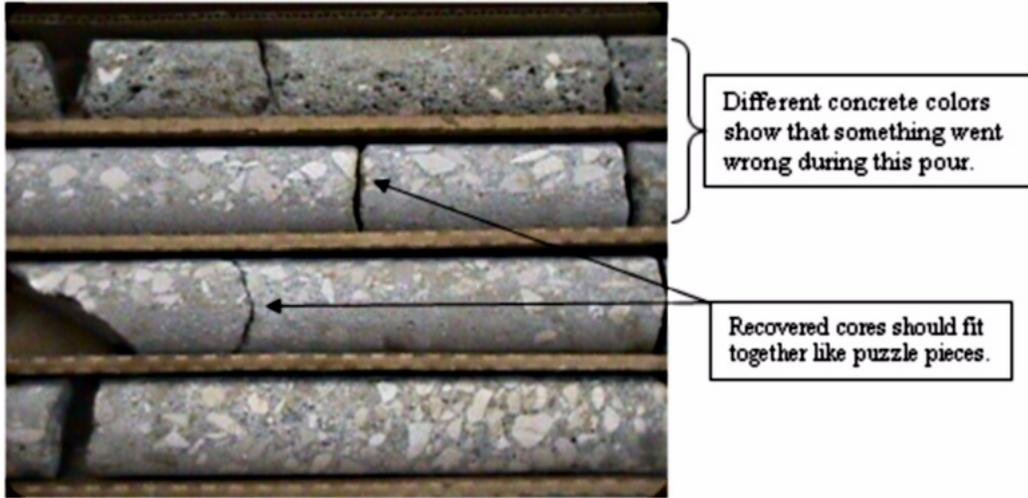
If a repair is required, at least one more hole will be required so that there will be an input hole and a return hole for cleanout and grouting. Do not core any hole more than 6” below the void. Coring below the void complicates cleaning out the hole.
