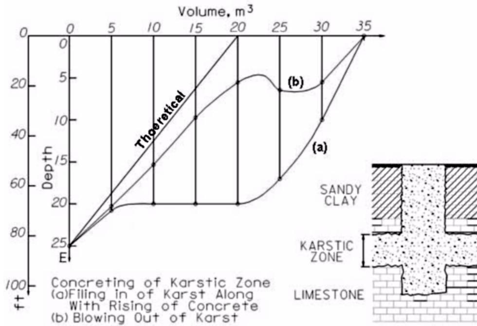
The above two graphics show the effects of subsurface conditions that may change the volume of concrete that is placed in the shaft. The above shows soft silts and karstic zones which require the actual concrete volume to be greater than the theoretical calculated volume.
