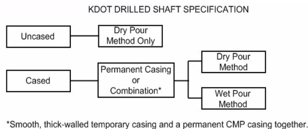
The previous graphic is a summary of the general type of excavations and methods of concrete placement; these are controlled both by plan call-out or in-field conditions.
