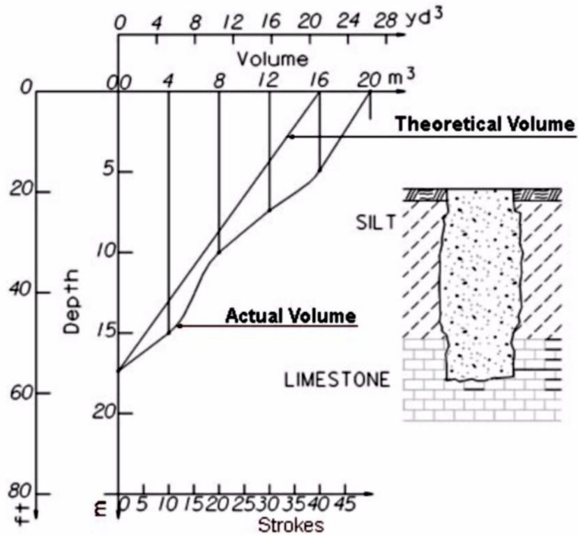
*Shafts with soft sidewalls may bulge slightly, requiring more concrete to be used.*
